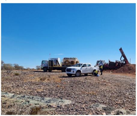
Figure 1: Aircore Drilling Rig at the Austin Gold Project
