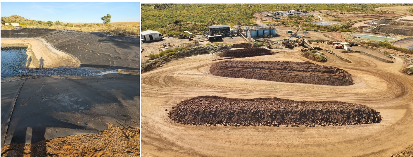
Figure 3: Copper in-solution from heap leach; Figure 4: Stockpiled oxide ore from Mt Norma on ROM pad
