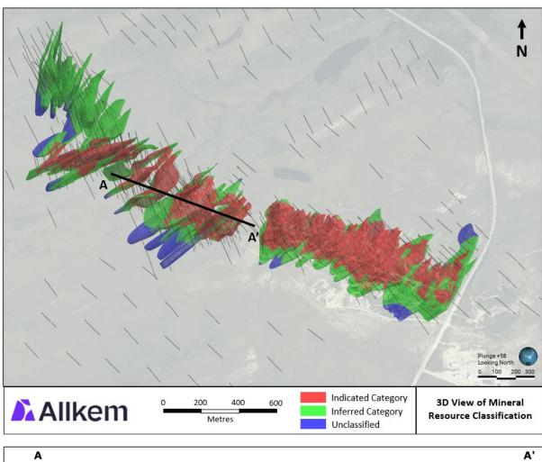
Figure 7: Isometric and section view (looking north) of the Mineral Resource Classification
