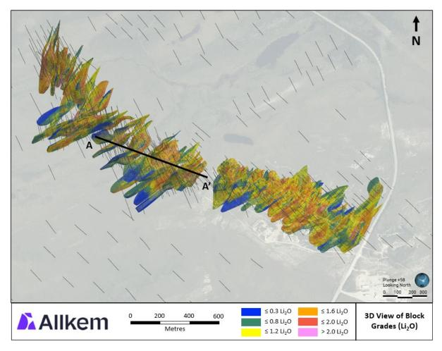
Figure 6: Isometric and section view (looking north) of Li<sub>2</sub>O Block Grades
