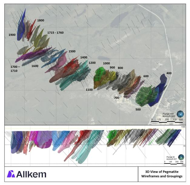
Figure 4: Isometric and section view (looking north) of modelled pegmatite dykes
