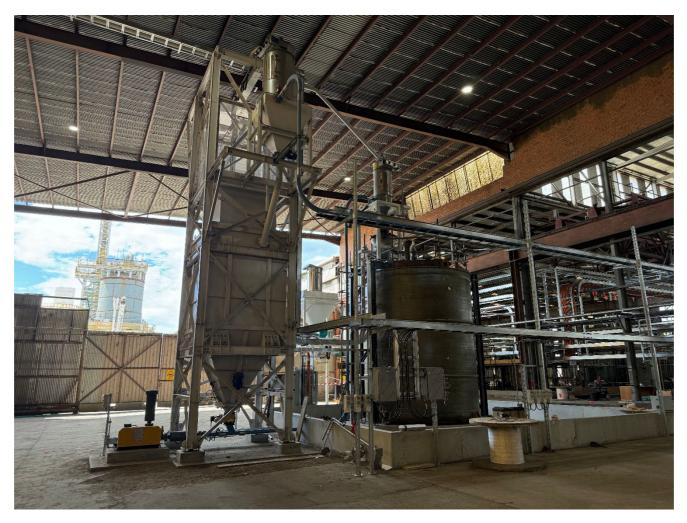
Figure: Magnesite Bag Breaker unit with pneumatics equipment installed
