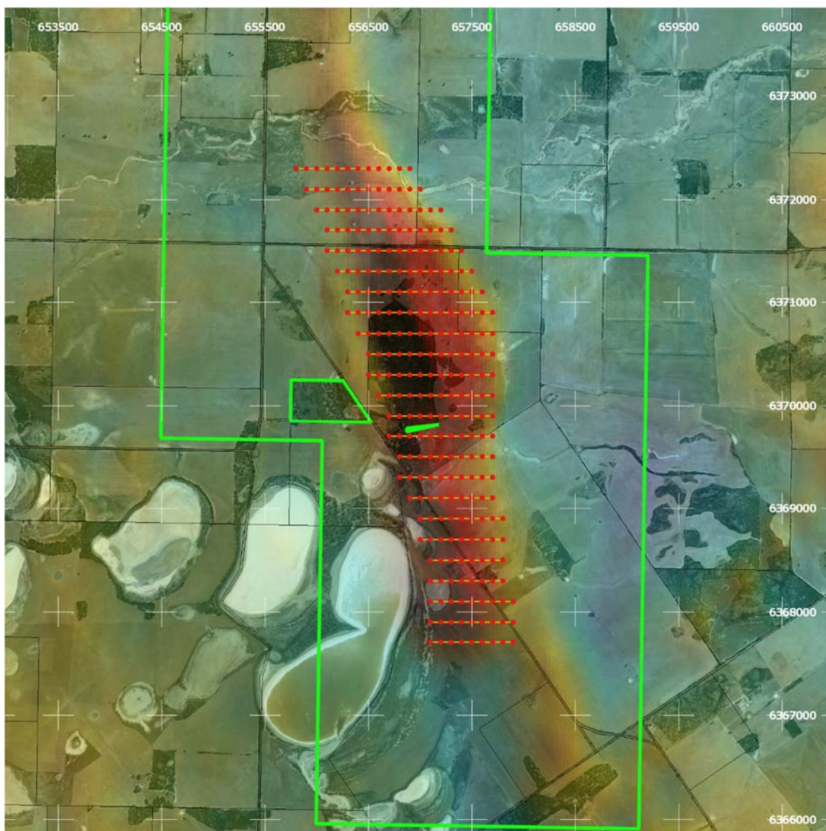
Figure 7 – Planned MLEM stations (red points) over satellite image with superimposed magnetic image
