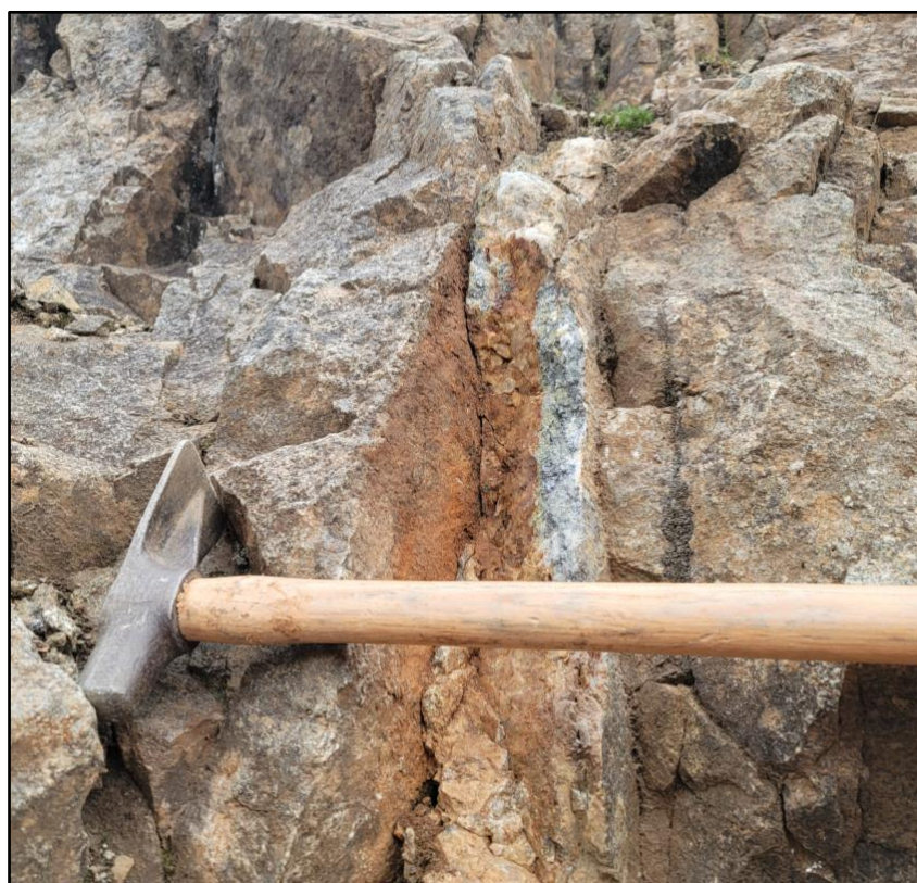
Figure 3. Sample E404601 – 90.5 g/t Au 9cm quartz-arsenopyrite vein
