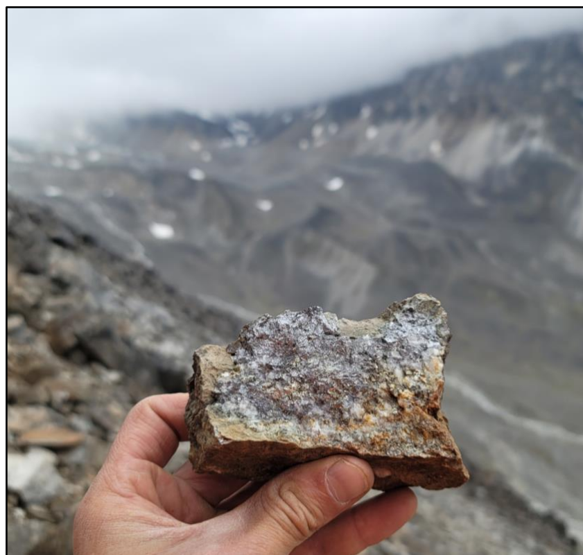
Figure 2. Sample E404605 - 127.5 g/t Au 7cm thick quartz-(70%)arsenopyrite vein with chalcopyrite. Southwest view of the upper tributary to Muddy Creek in background
