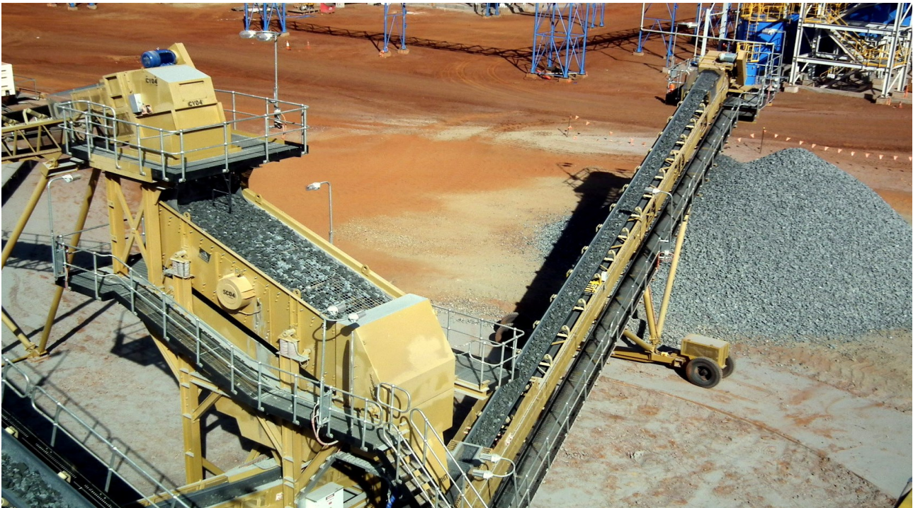
Figure 1: Scalping screen used for removal of the coarse (+40mm) native copper
