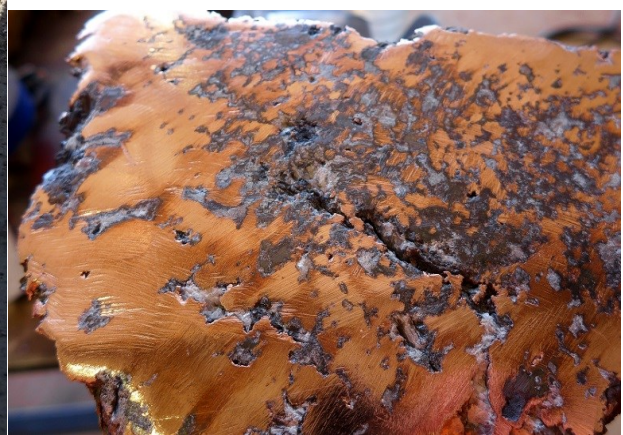
Figure 6: End piece cut from the above large nugget to create a base revealed near solid native copper metal (99.65% Cu), surrounding chalcocite (79.9% Cu), minor cuprite (88.8% Cu), and remnant minor calcite. This sample estimated at ~95% copper content by weight.
