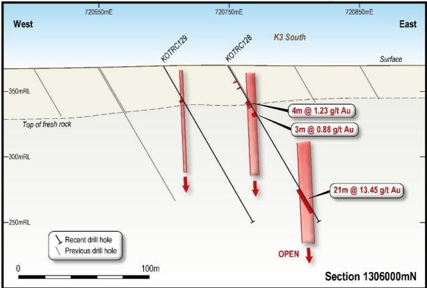
Figure 2. Section 1306000mN showing composite intercepts.
