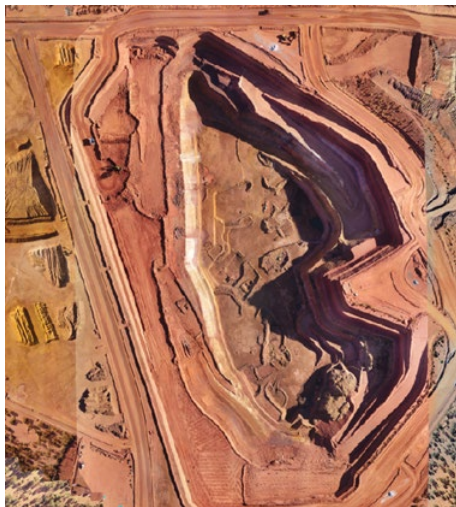
Mining Campaign 4-1 waste mining underway Western cutback of current pit
