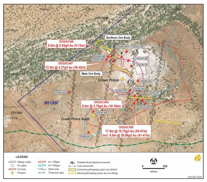
Figure 2. Significant air core drill holes intersections and the inferred extension of the mineralisation at Crown Prince
