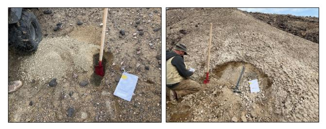
Figure 4. Sample location of anomalous lithium samples a. 721ppm Li (sample #1792531) and b. 699ppm Li (sample # 1792533).
