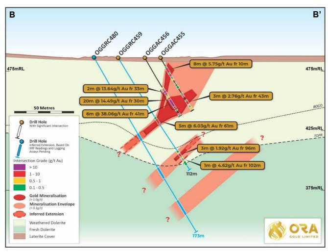
Figure 5. Down-dip gold intercepts and the inferred extension of the mineralisation (BB' cross-section)
