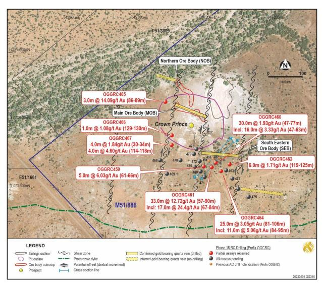
Figure 3. Recent drill holes intersections and the inferred extension of the mineralization at Crown Prince
