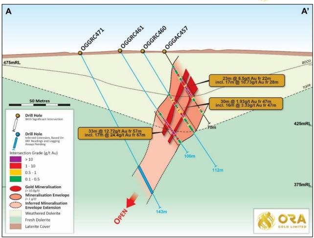
Figure 4. Down-dip gold intercepts on the SEB-Lode and the inferred extension of the mineralisation (AA' cross-section)
