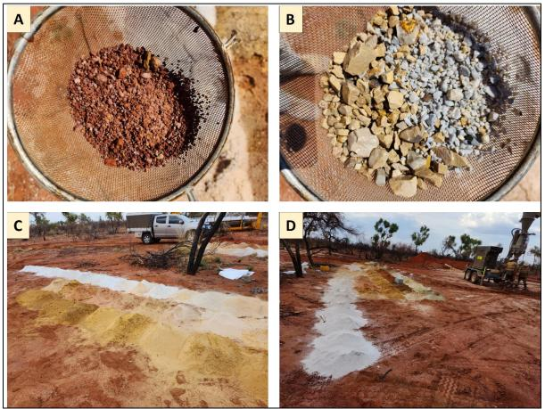
Figure 2: Geological variability of the Georgina Basin Sediments demonstrated by A: Highly oxidised lateritic clays, B: Chert and siltstones chips, C & D: Argillaceous sandy soils (orange/yellow) and highly sorted medium-grained sandstone (white).
