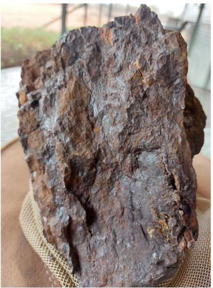
Figure 6: Photograph of the massive ironstone found at the Candy Colette Anomaly with abundant manganese and specular haematite.
