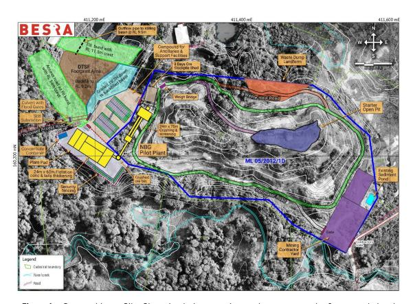
**Figure 1** – Proposed Jugan Pilot Plant site design, superimposed onto topography & grey-scale Landsat imagery.
