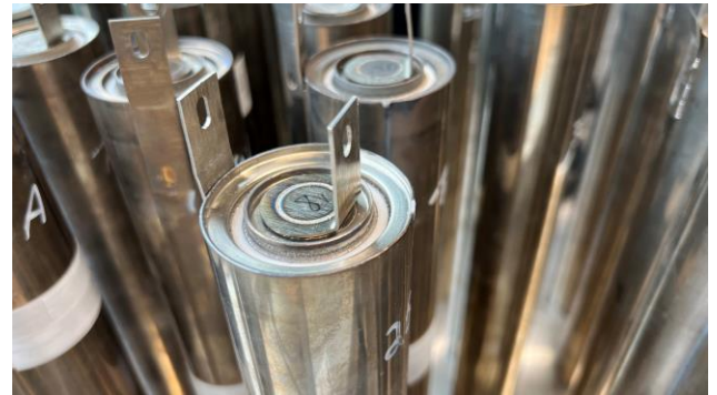
Figure 6 – CERENERGY® cell with positive and negative terminal
