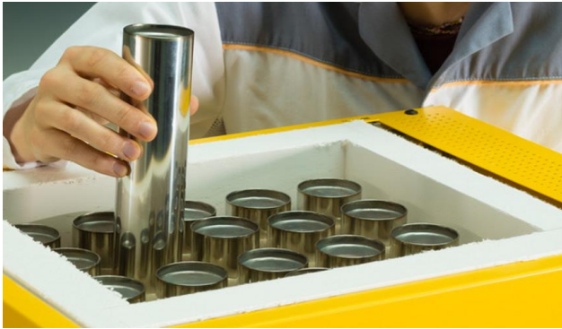
Figure 3 – CERENERGY® cells in battery module
