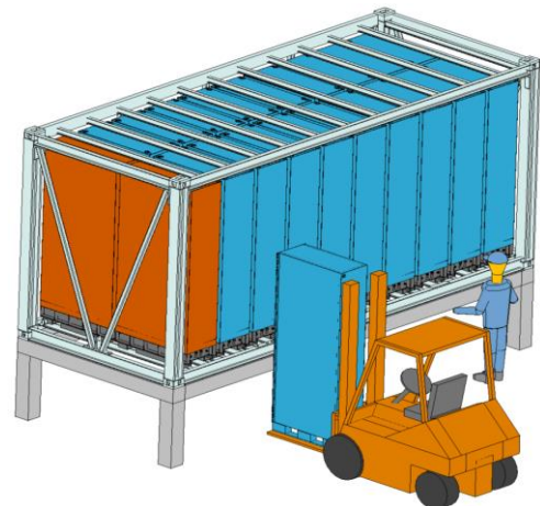
Figure 25 – Assembly 1 MWh GridPack
