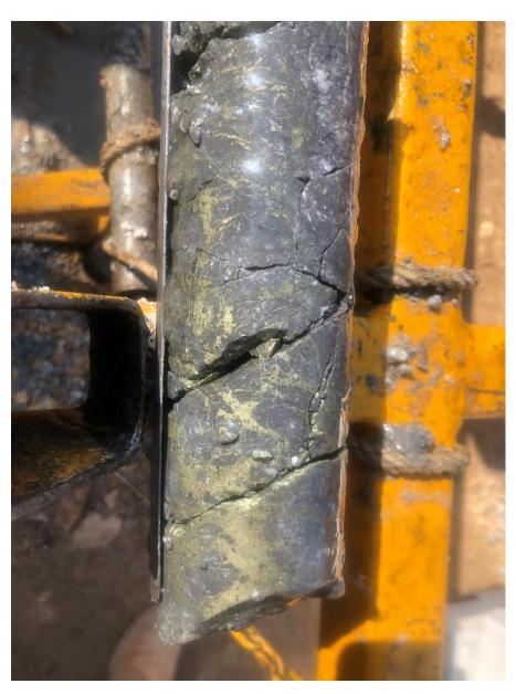
Figure 1. Chalcopyrite mineralisation within rhyolite porphyry, BWDD023 163m depth.
