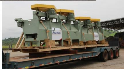
Denver 21 Flotation Cells delivered to the Project
