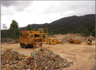
**Picture 14:** Primary crusher being transported to site.
