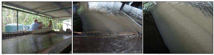
Pictures 8, 9 and 10: Gravity table trial with distinct separation of high and medium grade concentrates and waste.
