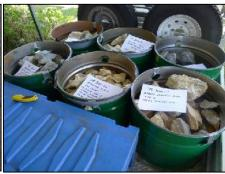
Pictures 11, 12 and 13: Excavation of bulk sample, size reduction and separation into various mineralisation types.
