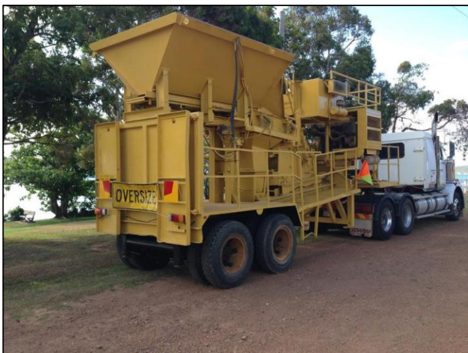
Picture 14: Primary crusher being transported to site.
