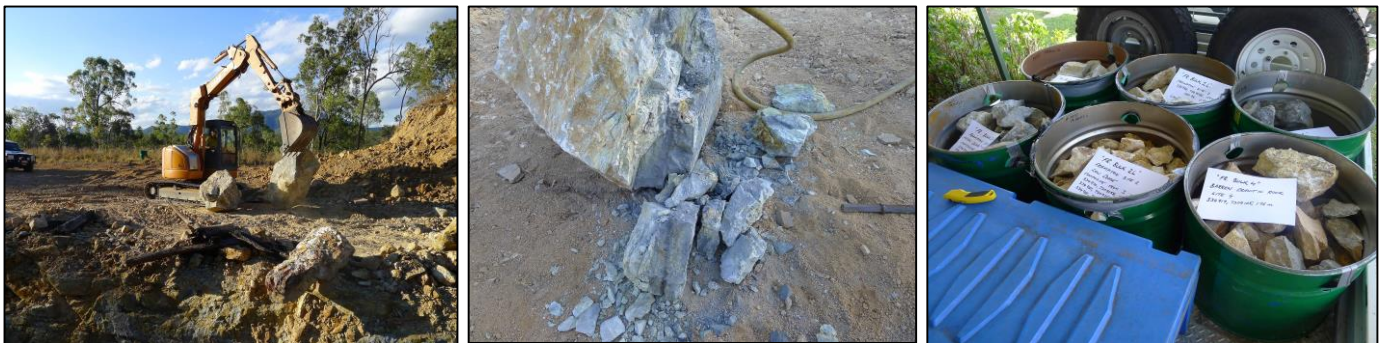
Pictures 11, 12 and 13: Excavation of bulk sample, size reduction and separation into various mineralisation types.
