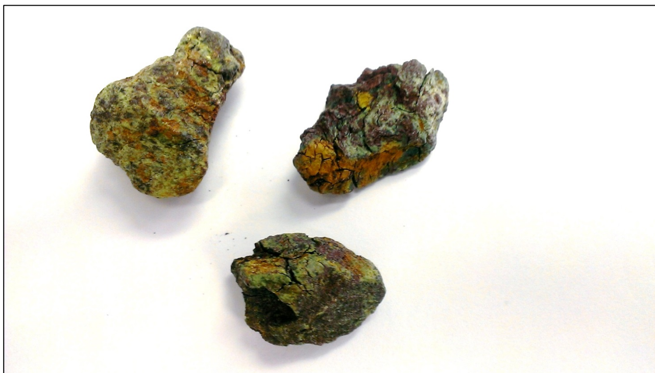
Figure 1: Nickeliferous gossan, containing the mineral gaspeite (Ni,Fe,Mg)CO 3 , from aircore hole FEAC278 at the Sabre prospect. Gaspeite is known from only a handful of locations worldwide. Aside from its type locality in Canada, gaspeite is found in the nickeliferous gossans of Kambalda type komatiitic nickel ore deposits in Kambalda, and nearby Widgiemooltha Townsite, both south of Kalgoorlie, Western Australia
