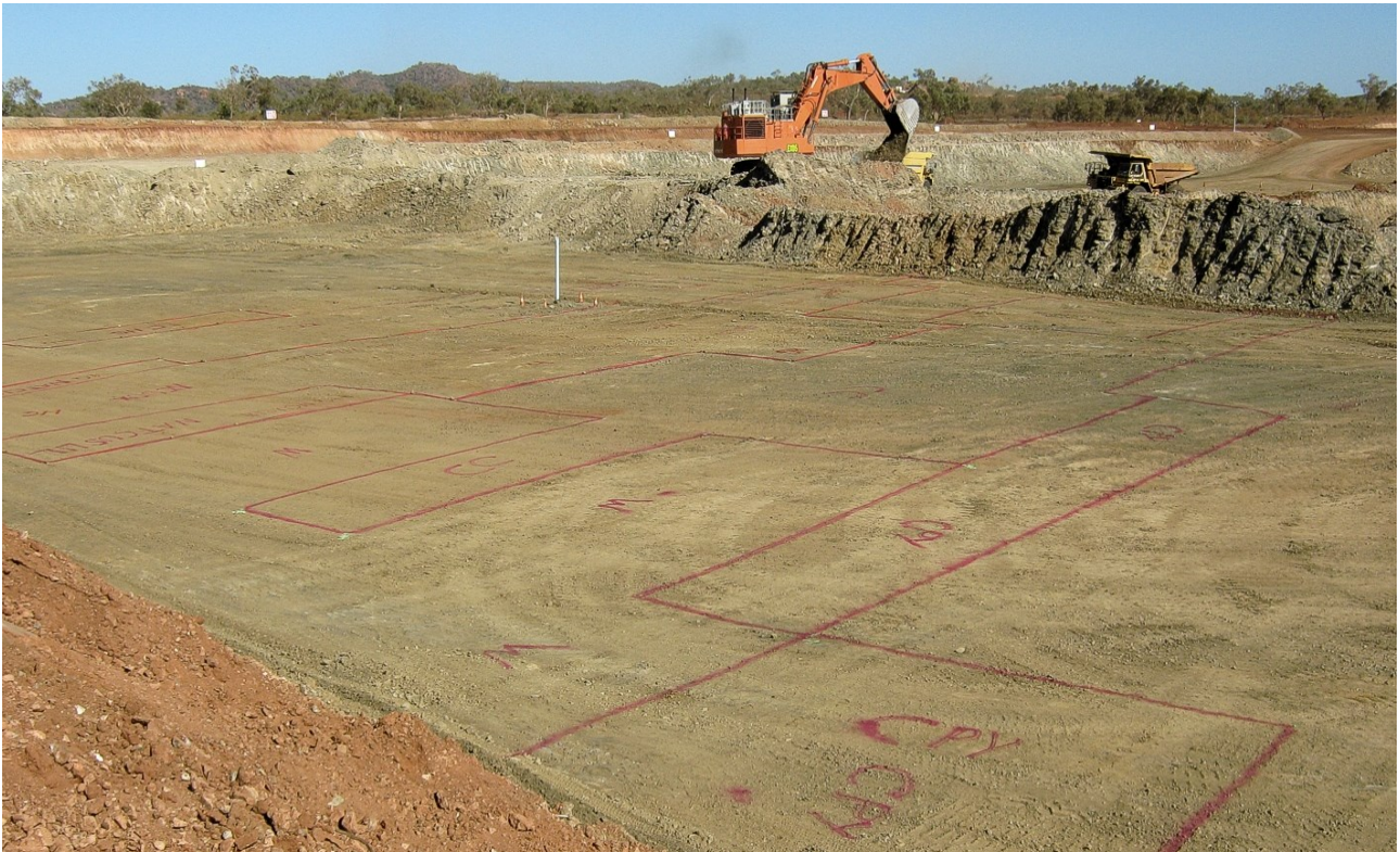
Figure 16: Pit mark-up at RL210 in a section of the Las Minerale starter pit. The areas marked include chalcopyrite (CPY), chalcocite (CC), native copper (NatCu), Oxide (Ox) and ore-based waste (W). In the middle stands a PVC drill collar from a decommissioned in-pit dewatering borehole. The ore zone is approximately 50m wide at this location.
