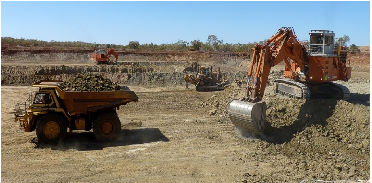
Figure 13: Mining has commenced in the LM Starter Pit. Waste was diverted to the complete the ROM pad which is now completed and ore is being sent to the stockpiles for later processing.
