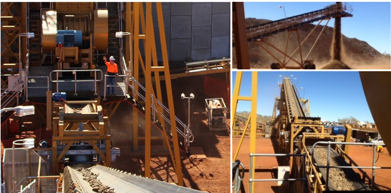
Figure 1: First few tonnes of ore to be crushed through the Rocklands Crushing Circuit - test-crushing of low-grade native copper oxide ore commenced today. Left image shows Executive Director Peter Hutchison overseeing proceedings.
