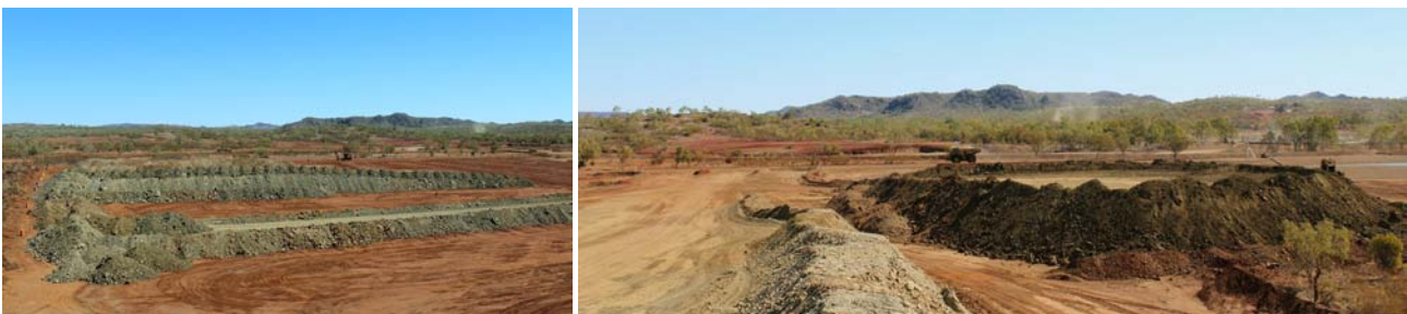
Figure 17: Stockpile inventory is building. Left; commissioning ore (left) including chalcocite, chalcopyrite and oxide ore types and right ; high-grade native copper oxide stockpile.
