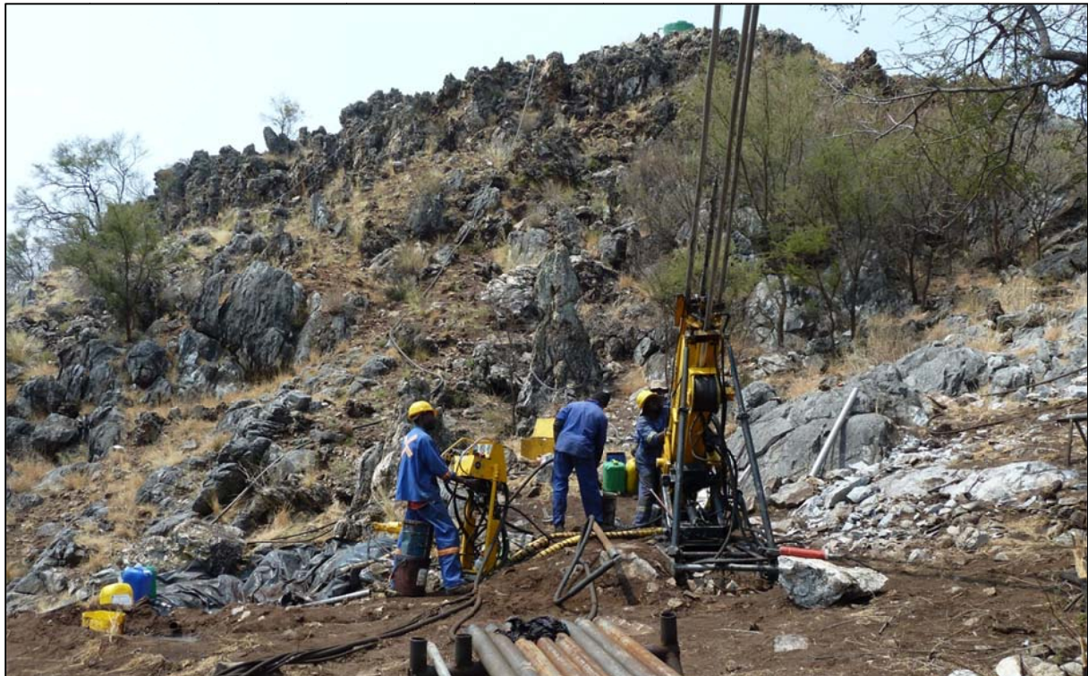
Figure 1 - Diamond drilling underway near the peak of the Eisernenhut, Otavi Mountain Land, northern Namibia.
