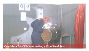
Still in PNG, a welder testing program for Clough Curtain JV was conducted at our facility in Clark during May. The testing consisted of various pipe welding tests in material sizes ranging from 50 – 450mm. To meet stringent quality requirement, a new electrode oven was purchased and a mobile dark room for x-raying test coupons was mobilised to the facility. This program was also followed up with welder testing for work at Darwin LNG and the Bayu Undan Gas Field.
