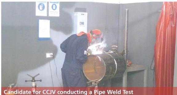
Candidate for CCIJ conducting a Pipe Weld Test
