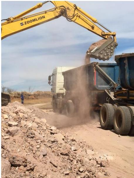
Figure 2. Trucks being loaded with ore
