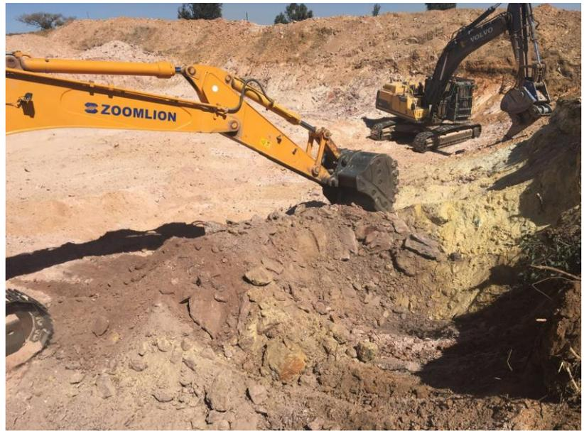
Figure 3. Ore being ripped and prepared for removal
