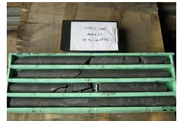
Strongly weathered graphitic schist below BOCO. Graphitic schist progressively more competent with depth. 11
