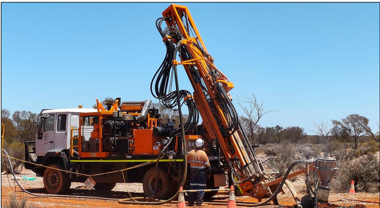
Figure 1 - Rainbow Dam RC drilling - Photo courtesy of Salazar
