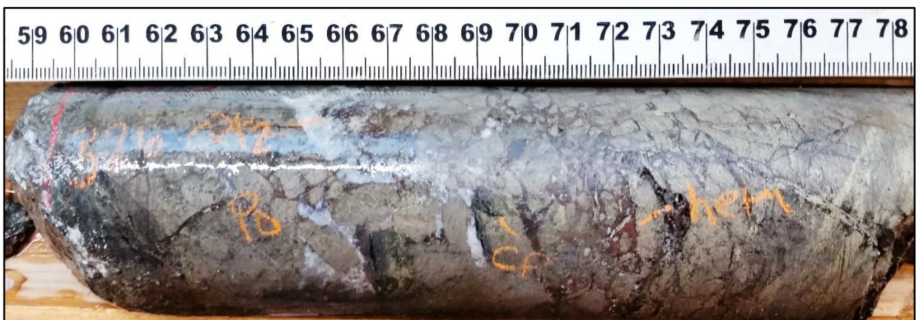
ZA-19-03: 52m - Massive Sulphide comprising pyrrhotite-pyrite-chalcopryite in a quartz breccia
