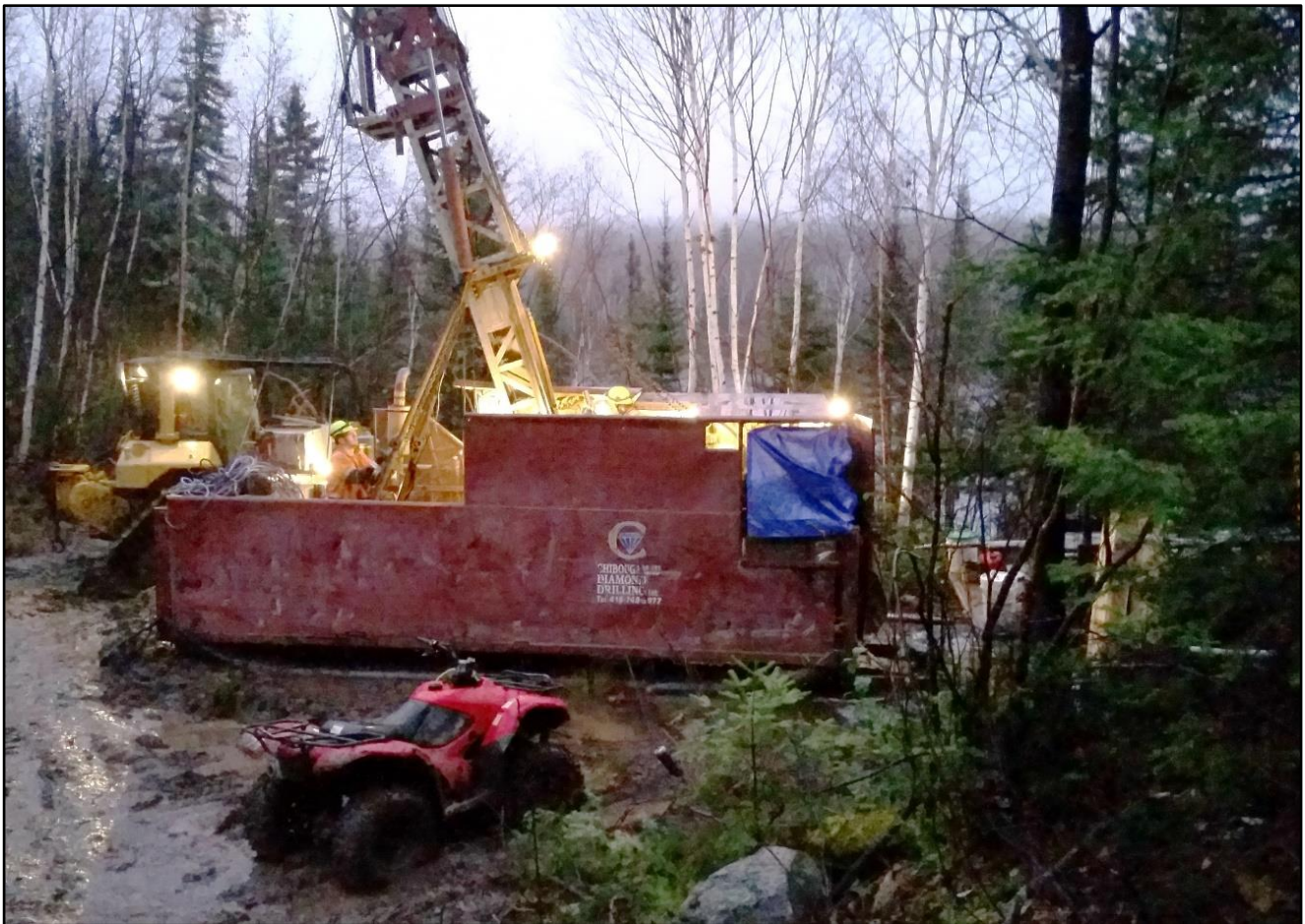
Chibougamau Diamond Drilling Ltd (CDD) diamond drill set up on Alotta hole ZA-19-03
