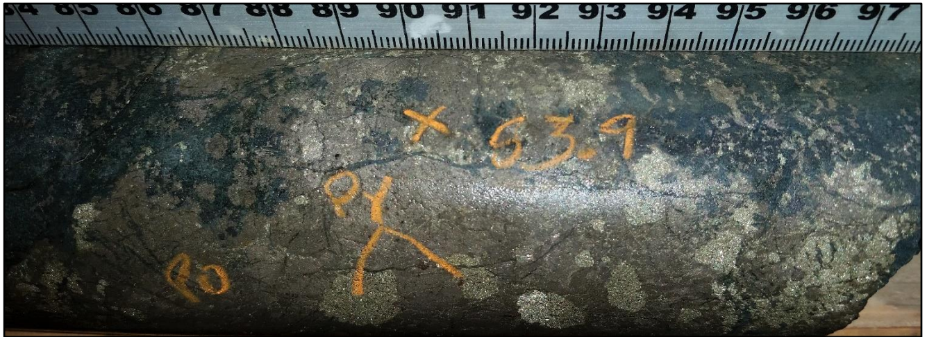
ZA-19-03: 53.9m - Mineralised gabbro with massive pyrrhotite and pyrite porphyroblasts
