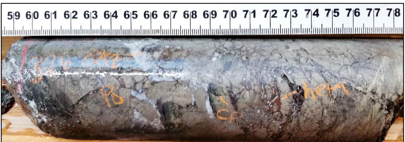
ZA-19-03: Massive Sulphide - pyrrhotite-pyrite-chalcopyrite in a quartz breccia at 52m downhole
