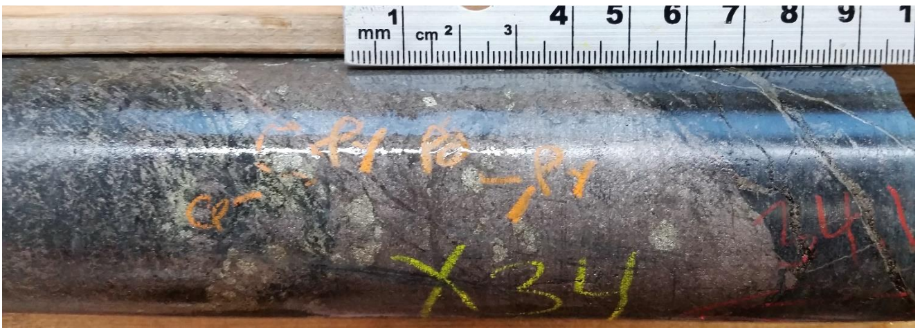
ZA-19-03: 34m – Gabbro with disseminated – net-textured massive pyrrhotite + pyrite
