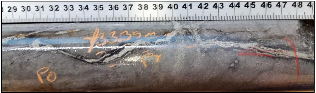
ZA-19-03: 33.35m – Gabbro with remobilised massive pyrrhotite + pyrite
