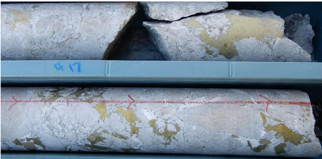
High grade copper in hydrothermal infill breccia CAE hole # 17, : 404m depth. Interval 404m-407m : 3m @ 1.85% CuEq, 1.52% Cu ,0.31 g/t Au,17.2 g/t Ag.
