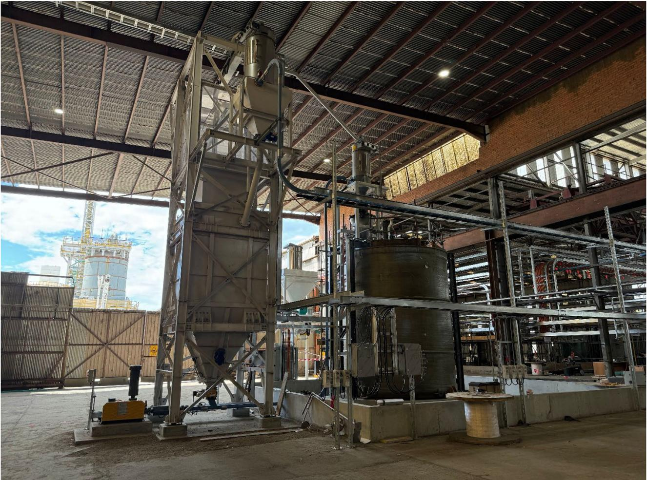
**Figure:** Magnesite Bag Breaker unit with pneumatics equipment installed
