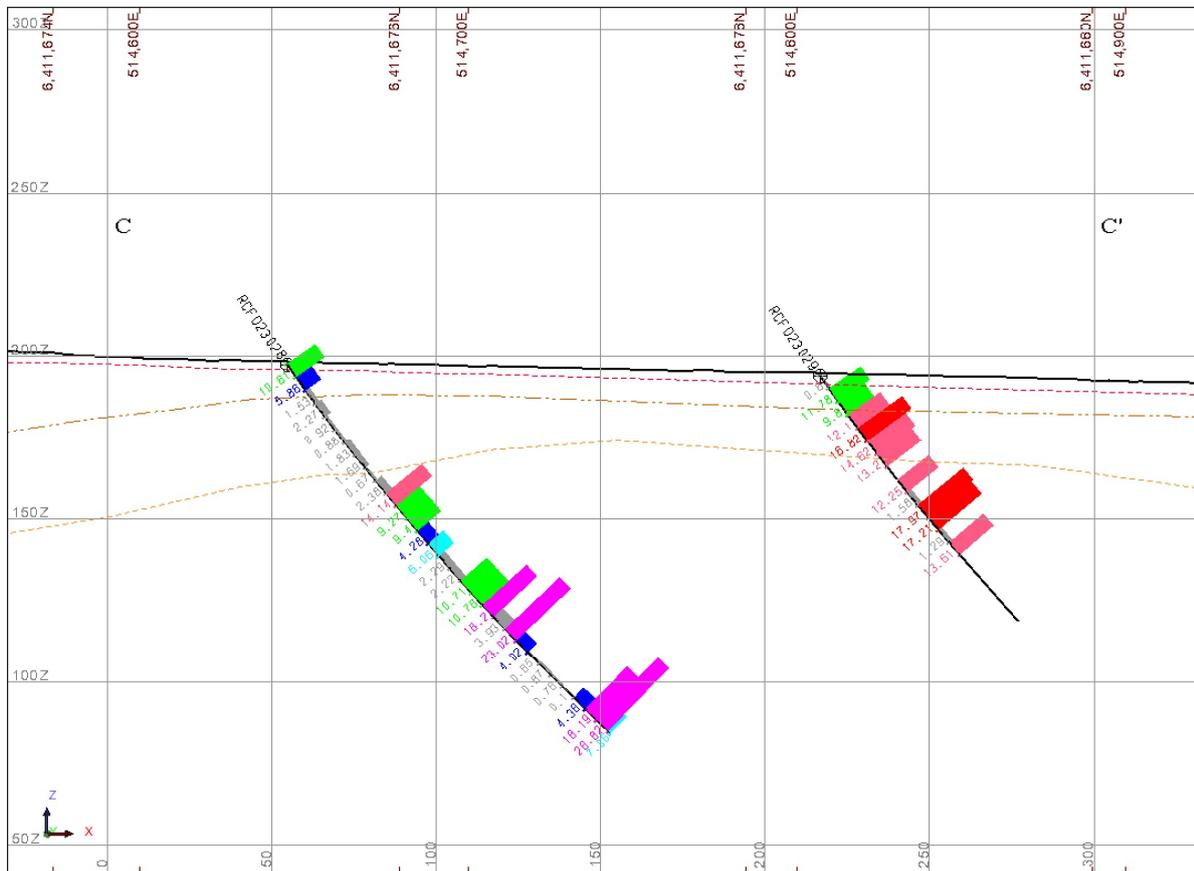
Figure 19: Drillhole Section C:C' RCFO23028 & RCFO23029 DTR%.
