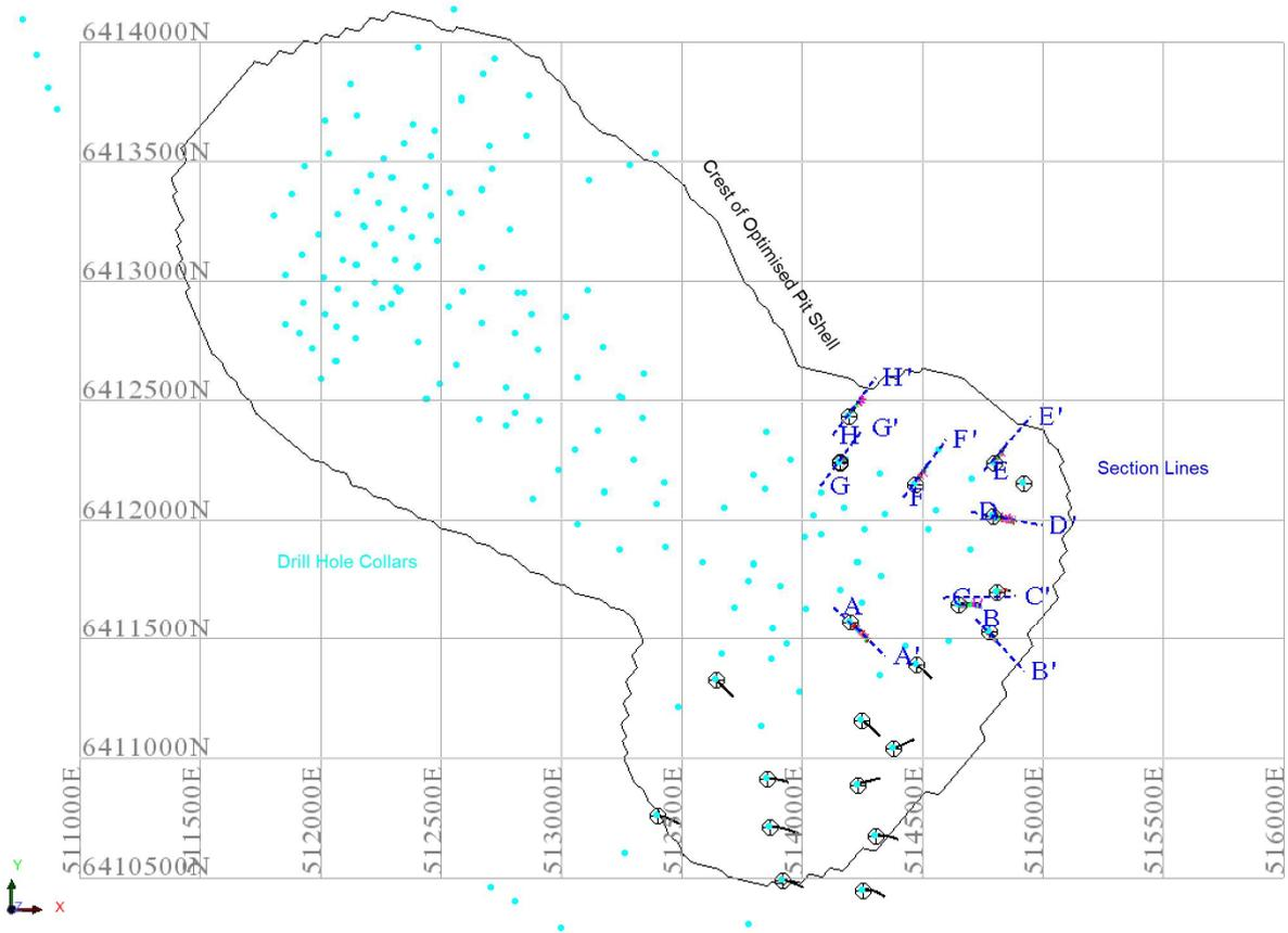
Figure 13: Location plan showing drillhole collars and section lines associated with the DTR sections below.
