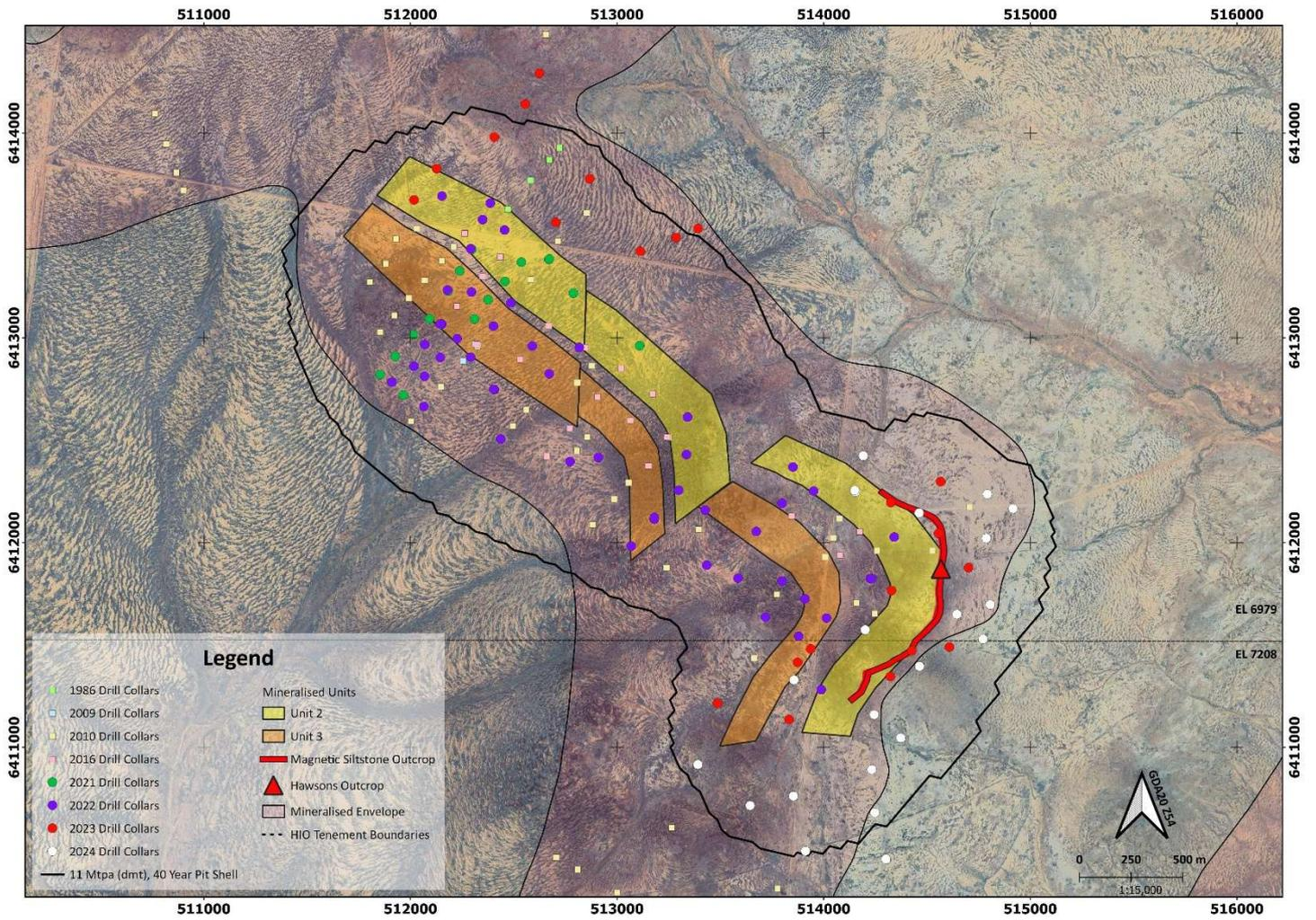
Figure 10: Drillhole location plan within the resource area showing potential modelled units of mineralization (yellow) and potential faulting. The pink zone indicates the extent of the interpreted magnetic anomaly (TMI RTP). Drillhole locations shown are historic holes up to 2021-22 and recent 2023 & 2024 drillholes.
