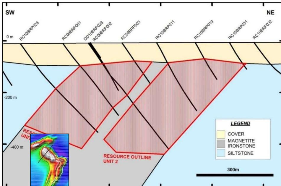
Figure 11: Generalised NE-SW cross-section through the Core West area showing the dipping sediments and core intersections from previous drilling (source: CAP, 2010).
