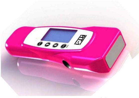
Figure 5: CorMaGeo RT-1 magnetic susceptibility meter
