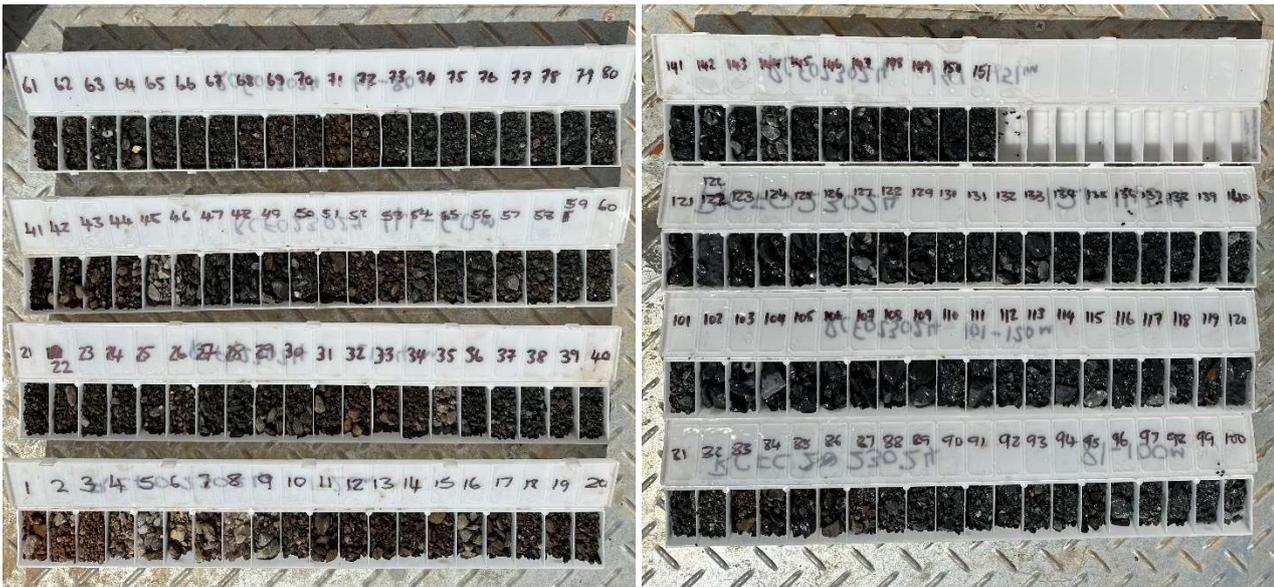
Figure 6: Photo of RC sample chips: Drillhole RCFO23024, 1-151m (TD).
