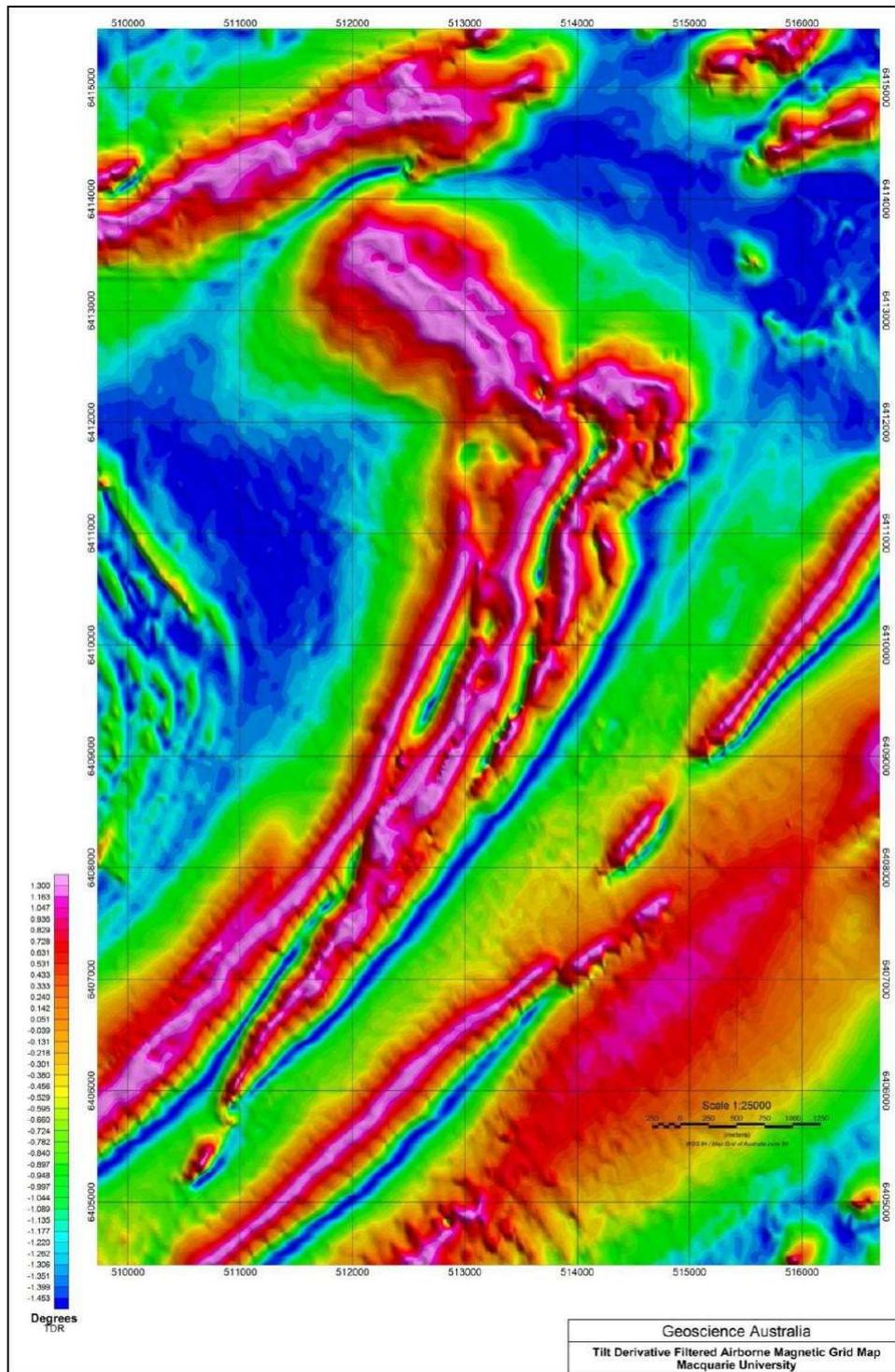
Figure 12: TMI RTP - Tilt Derivative Filtered Airborne Magnetic Image of the Hawsons Iron Deposit (after Camille R, 2012).
