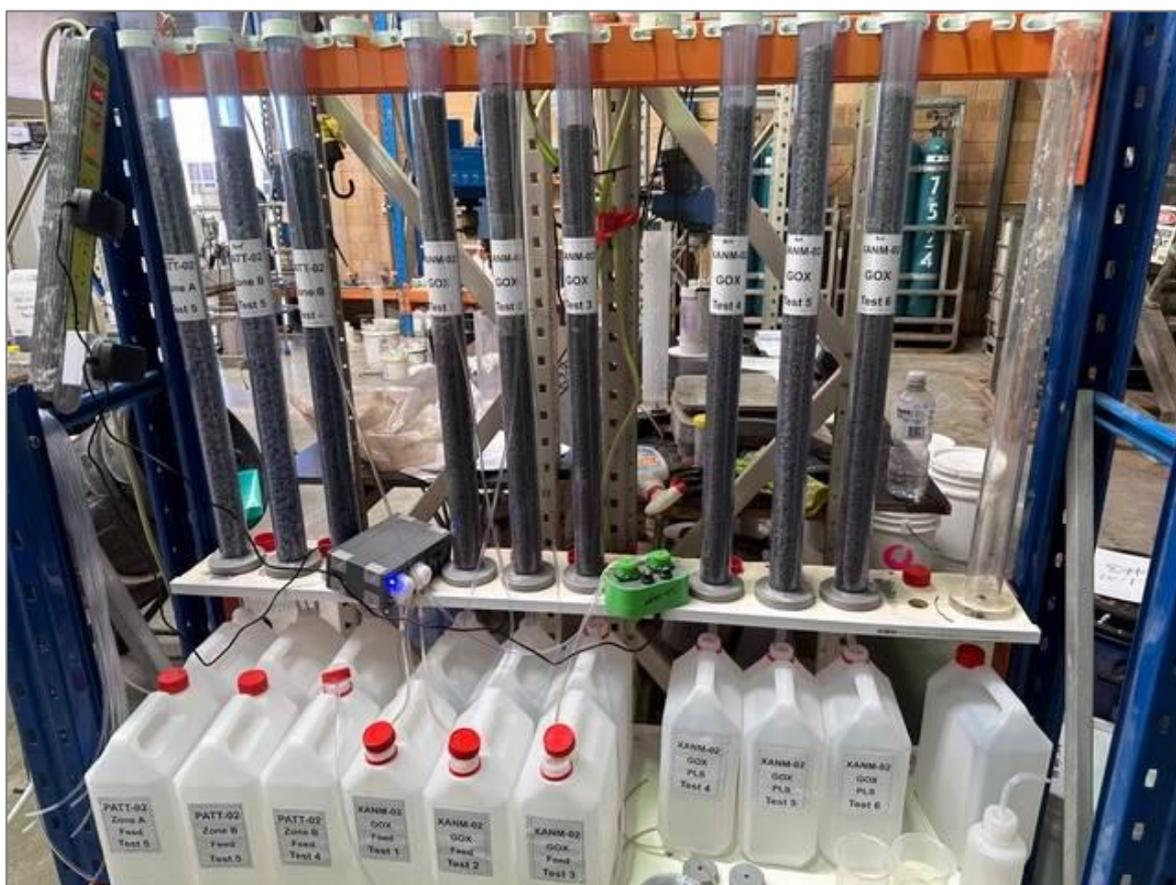
**Figure 1. Oxide Column Leach at DMPS Labs**
