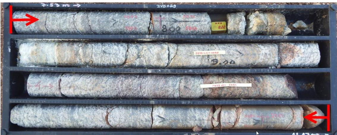
Figure 5: Oxidised graphitic gneiss (approximately 10% TGC) between 7.5 and 11.2m downhole in IVD029
