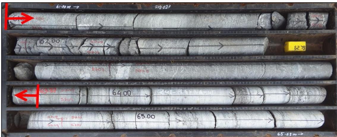
Figure 4: Graphitic gneiss (approximately 9% TGC) between 61 and 63.8 m downhole in IVD027
