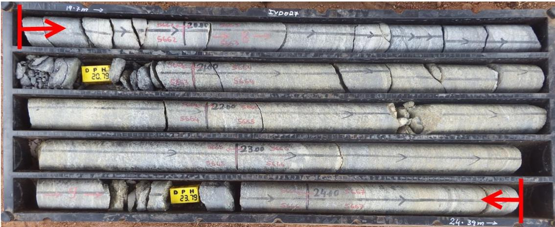
Figure 3: Graphitic gneiss (approximately 9% TGC) between 19.7 and 24.4 m downhole in IVD027
