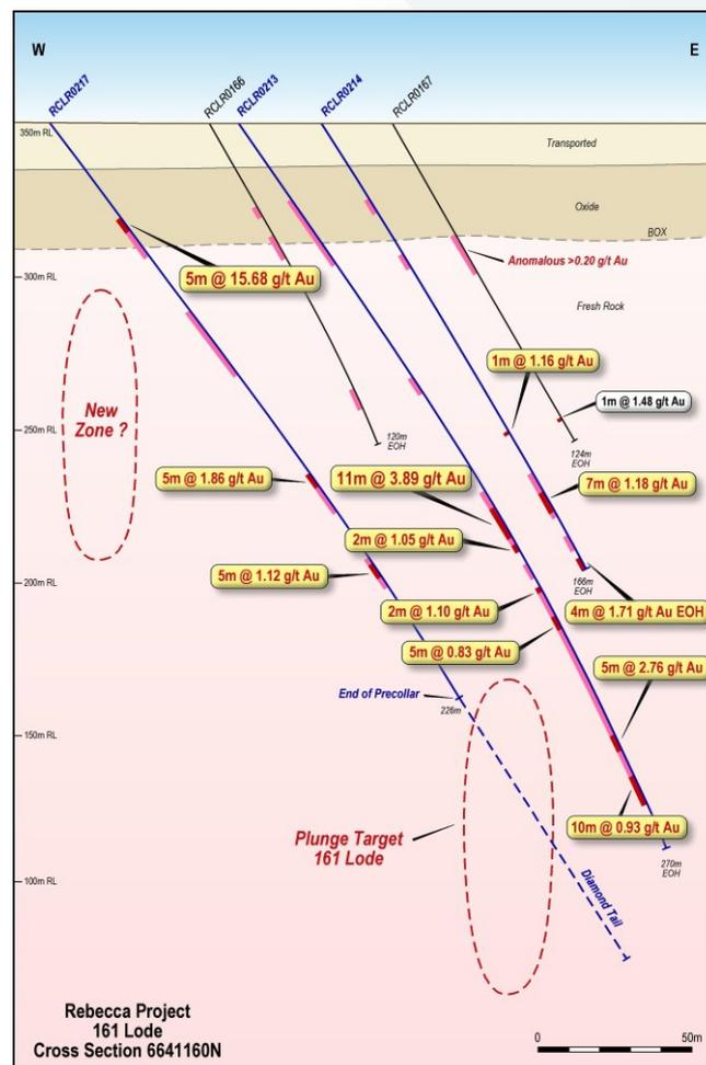
The 11m @ 3.89g/t Au intercept in RCLR0213 sits ~100m above an interpreted south-plunge position of the 161 Lode, a target that will be tested by diamond drilling from precollar hole RCLR0217 (Figures 2 & 3).
