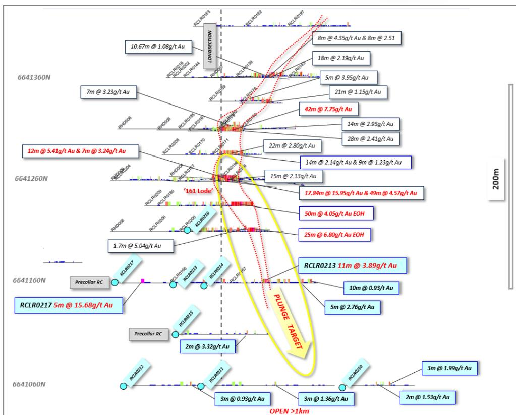
Drilling was carried out on three 50m spaced traverses at the southern end of Bombora, with eight holes completed of between 150m and 270m in depth. All drillholes intersected >1g/t Au disseminated sulphide-hosted mineralisation, typically within broad zones of >0.20g/t Au gold anomalism (Table 1).
