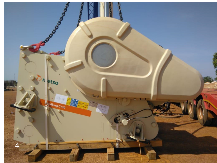
2 Pre-leach thickener foundation 4 C130 Metso jaw crusher delivered to site fully assembled
