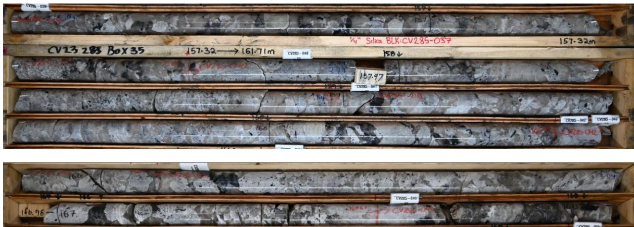
Figure 6: Centimetre to decimetre size spodumene crystals with feldspar and smoky quartz in drill hole CV23-285, at approximately 156 m to 161 m depth (TOP) and 166 m to 168 m depth (BOTTOM), grading 3+% Li 2 O over the respective interval.
