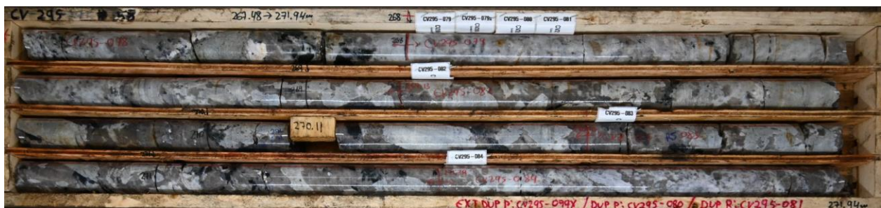
Figure 8: Centimetre to decimetre size spodumene crystals with feldspar and smoky quartz in drill hole CV23-295. From 269.1 m to 271.4 m core grades 3.4% Li 2 O.
