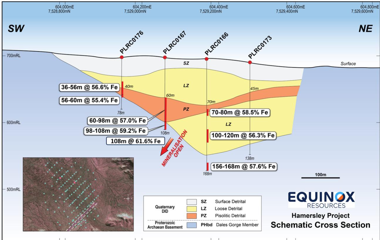
Figure 2: Cross-section of the higher grade near surface iron ore<sup>2</sup>.
