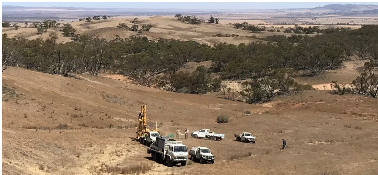
Figure 7: Aircore drilling at Walloway.
