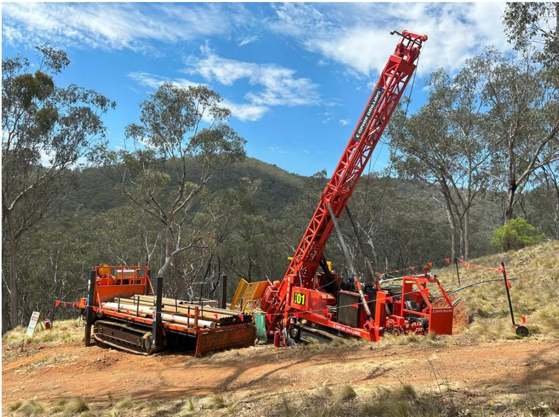
**Figure 1:** Diamond drilling at the Queenslander Deposit December 2023
