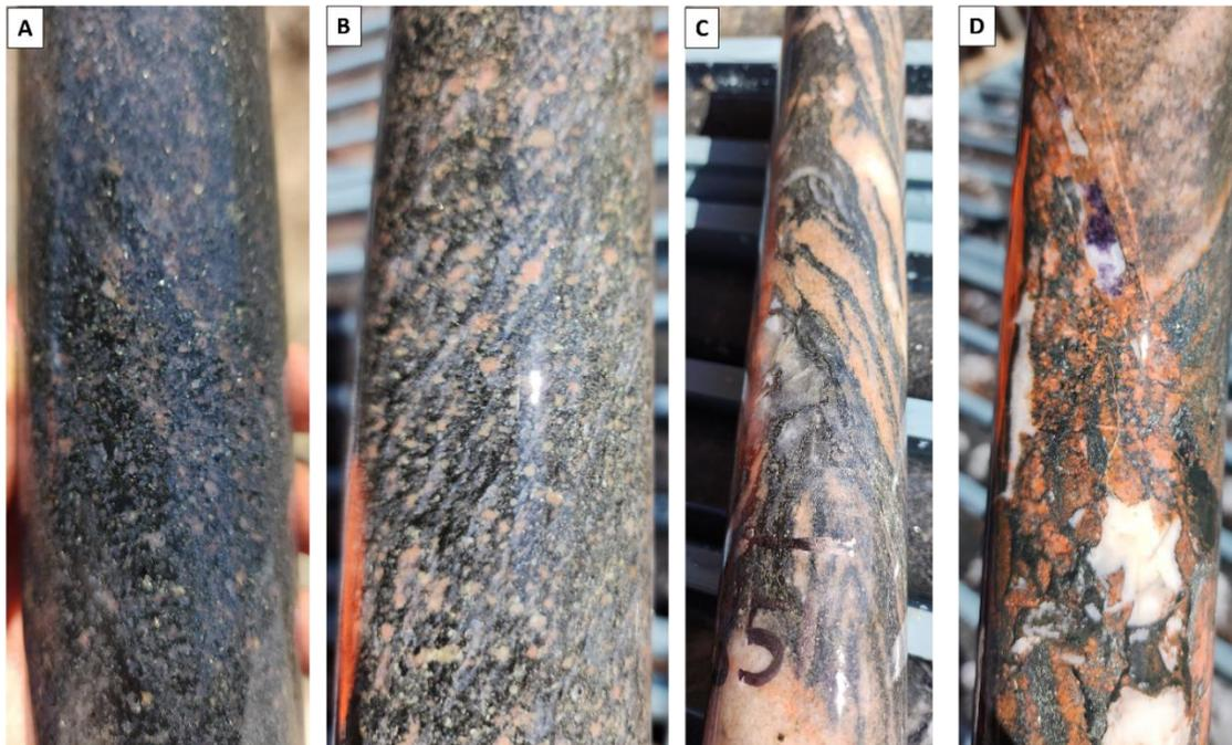
*Figure 1, Part 3: Core photo collage showing the progression of geology, alteration, and mineralisation. A: Altered granite with intense biotite alteration and disseminated sulphides at 525m, B: Altered granite with minor foliation and disseminated sulphides at 537m, C: Foliated and metamorphosed granite with quartz veins at 565m, D: Brecciated granite with quartz veining, fluorite infill and disseminated sulphides at 570m.*
