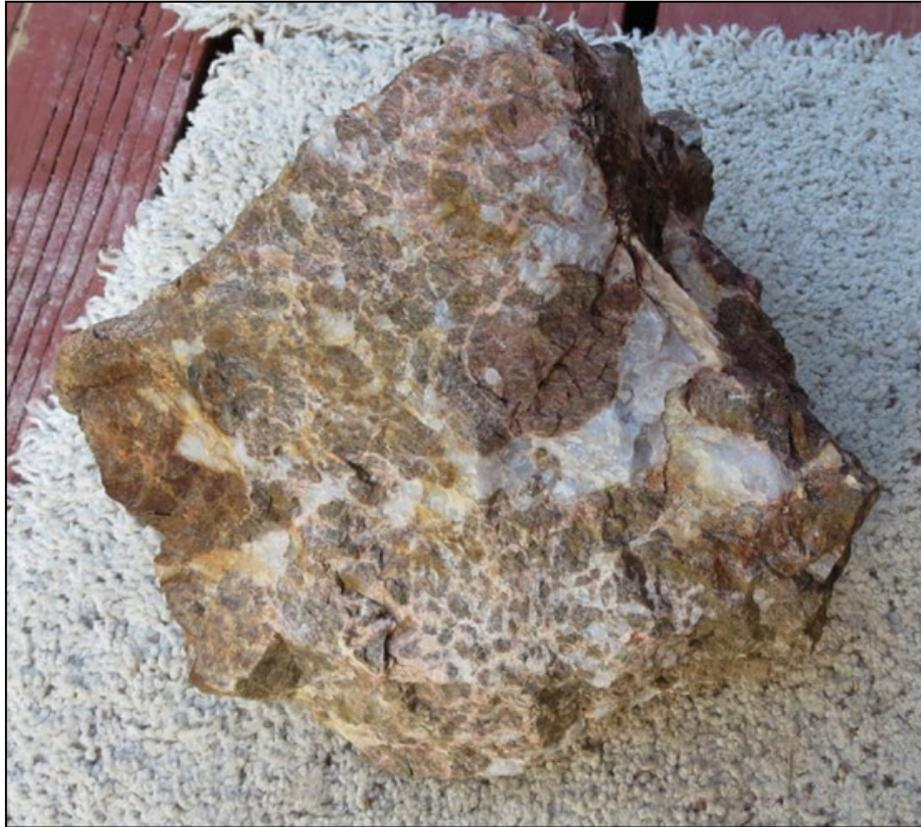
*Photo 2 – Field sample of brecciated pegmatite dyke collected from the Silver Dollar mine showing widespread pink potassic alteration.*
