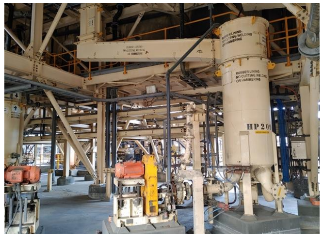
FLOTATION GROUND FLOOR TANKS AND PUMPS
