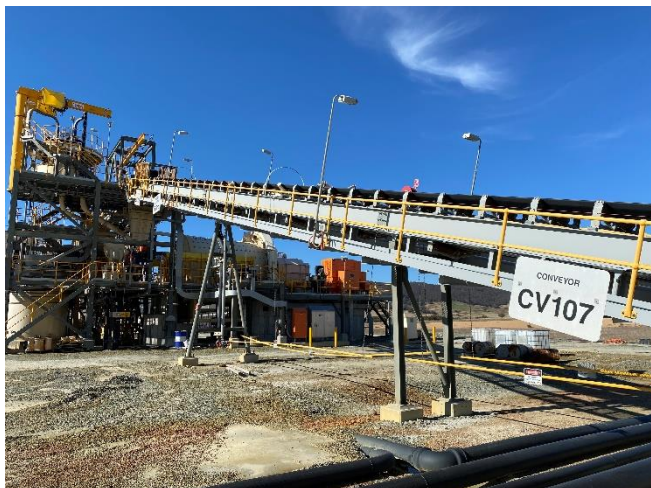
CONVEYOR FROM ORE BIN TO BALL MILL
