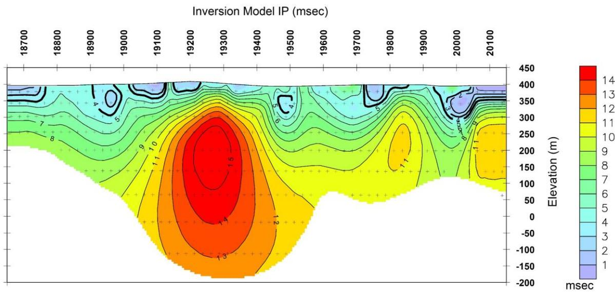
**Figure 6. IP line L4900E Inversion Model Chargeability Section.**
