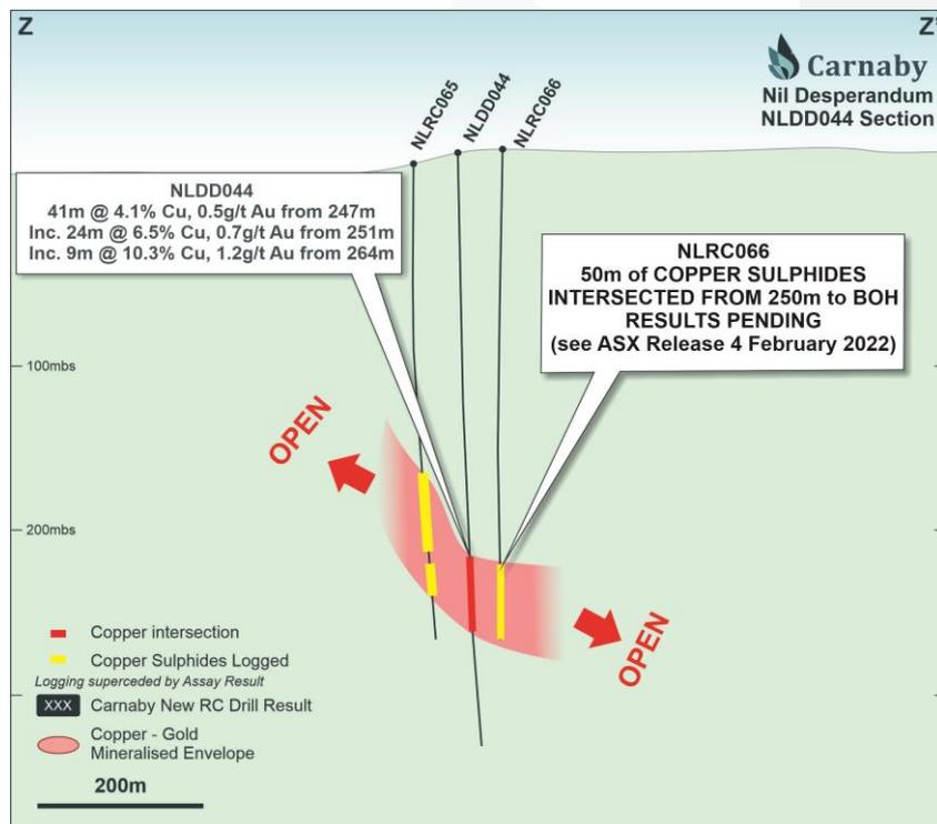
Figure 3. Drill Section showing location of drill hole NLDD044 and NLRC066.
