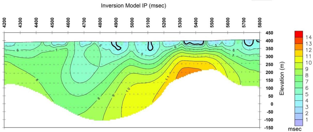
Figure 6. IP line L18500N Inversion Model Chargeability Section.
