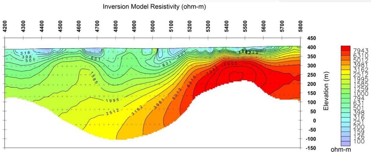
Figure 7. IP line L18500N Inversion Model Resistivity Section.
