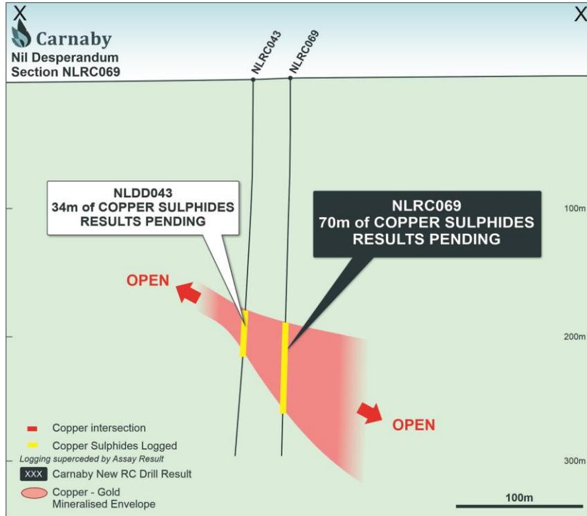
Figure 2. Drill Section showing location of drill hole NLRC069.
