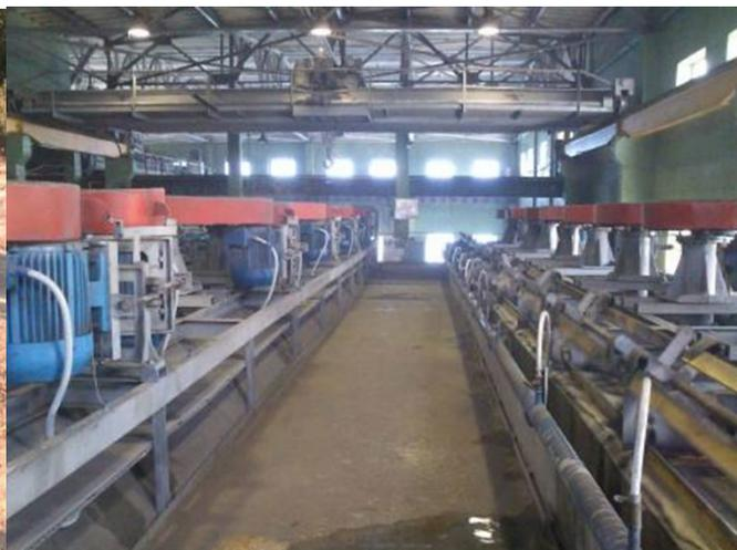
**Final stage flotation cells**
