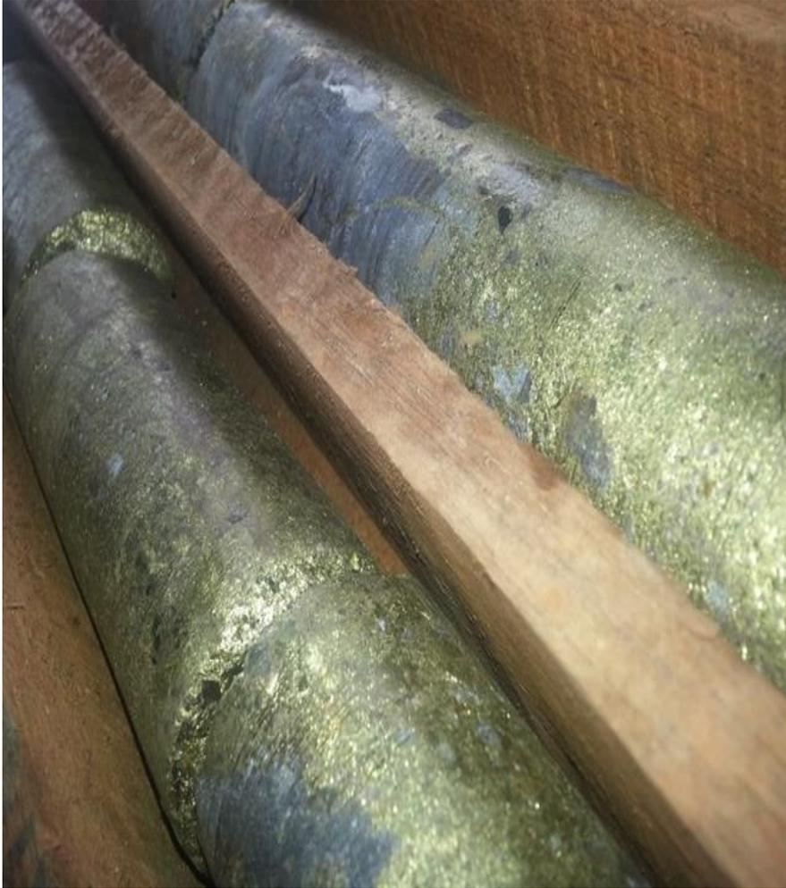
*Massive sulphide copper mineralisation*
