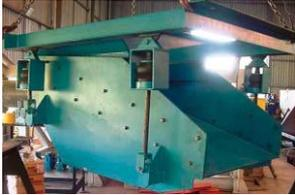
Simplex Vibrating Feeder being fabricated in Brazil
