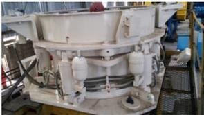
Mainframe of Avanco’s secondary crusher being assembled in Brazil
