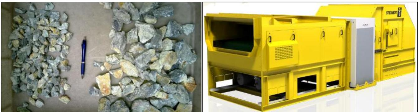
**Pictures 6 and 7:** The shear material sized for sorting and a typical Steinert X-ray Sorting System (XSS) machine.
