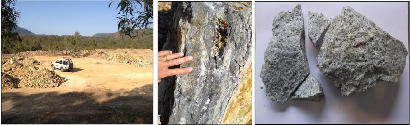
**Pictures 3, 4 and 5:** Frampton stockpiles, typical grade carrying shear material and typical barren wall rock.
