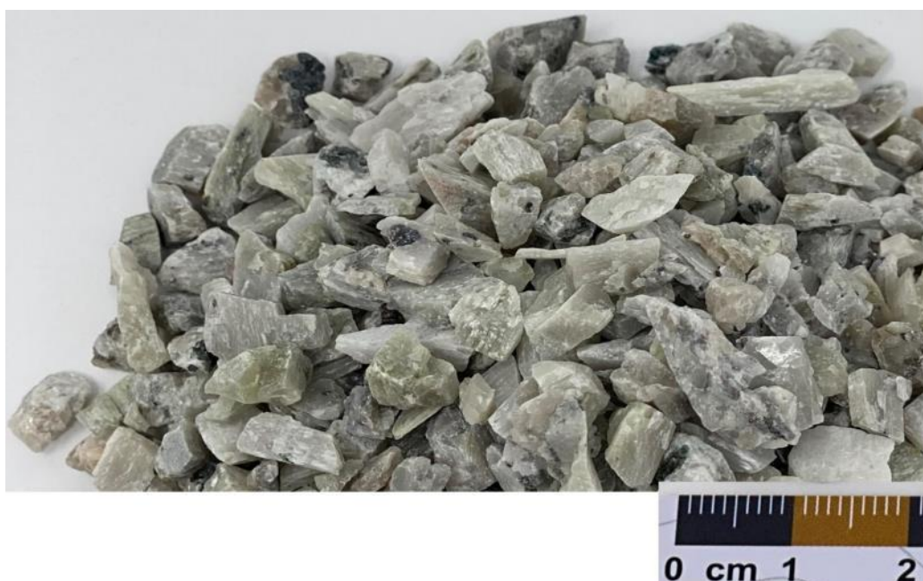
Fig 18 Spodumene concentrate produced from DMS test work
