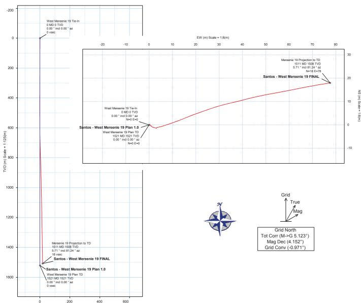
Vertical Section (m) Azim =  $0^{\circ}$  Scale = 1:125(m) Origin = 0N/-S, 0E/-W
