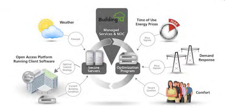
Machine learning technology - automatically learns and models a building's thermal characteristics and usage patterns Continuously obtains data on weather forecasts, realtime electricity prices, and DR signals Runs thousands of simulations to arrive at the most efficient HVAC operating strategy for the next 24 hours
